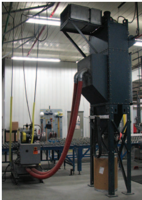
▲ Glass, aluminum carbide, and silicon carbide dusts are collected with the GS2.
