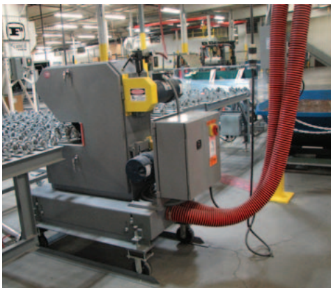
▲ High speed belts trim sharp edges at this unit.
