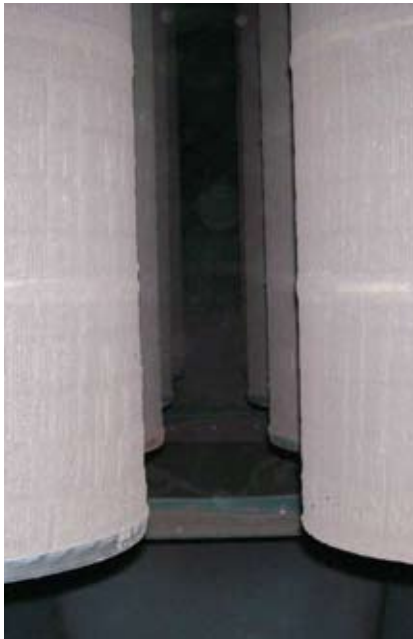
These filter pleats are plugged full of dust.
