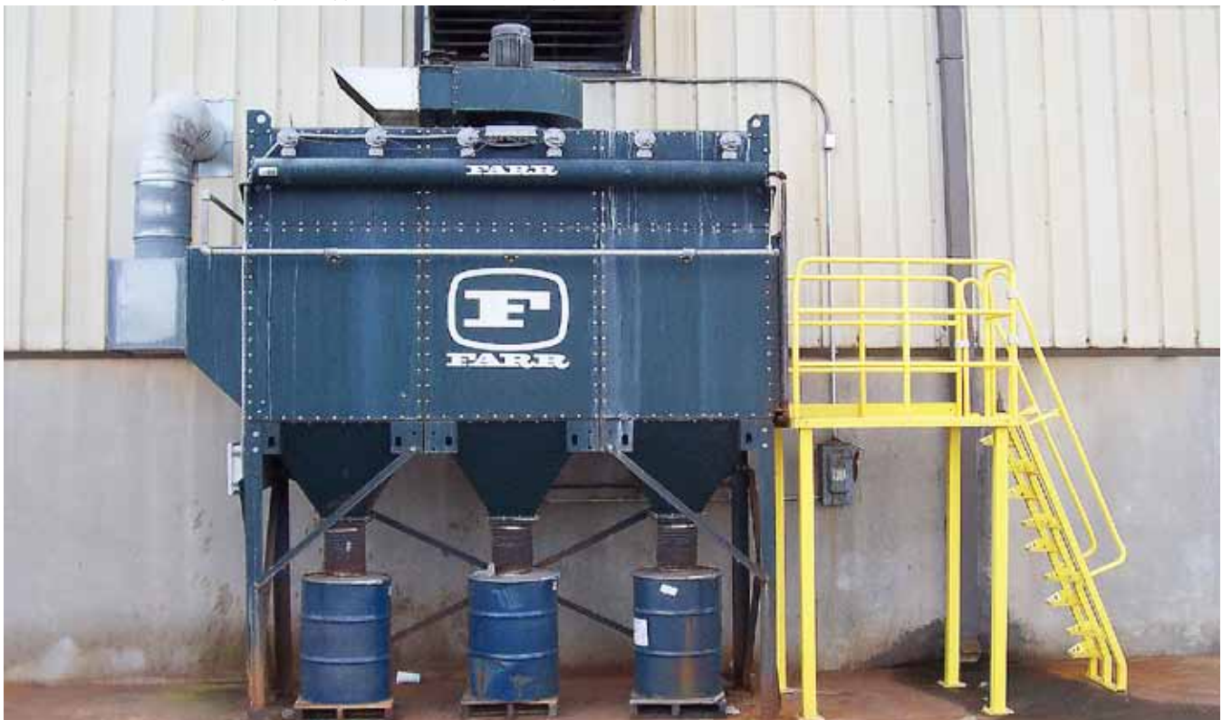
GS12 at Lapeyre Stair in Harahan, LA. on a metal shot blast application
