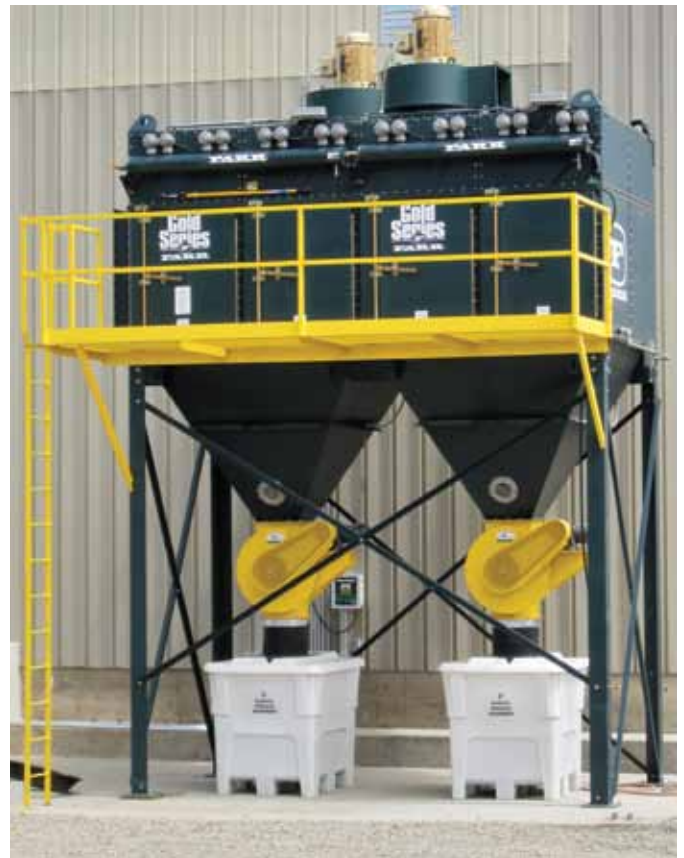
Gold Series model GS32 collecting hay dust from presses.
