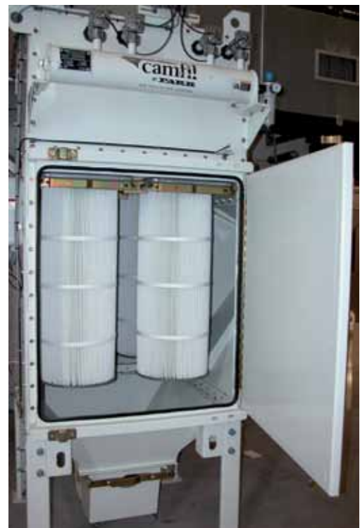
The Durapleat Gold Cone cartridges fitted to the units are a washable, heavy-duty spun-bond polyester, providing high efficiency filtration, with a low pressure loss and excellent cleaning characteristics for a long life.
