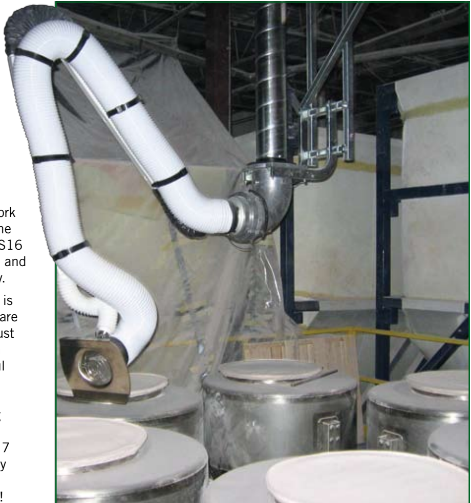
Food grade extraction arms being used with the GS16.
