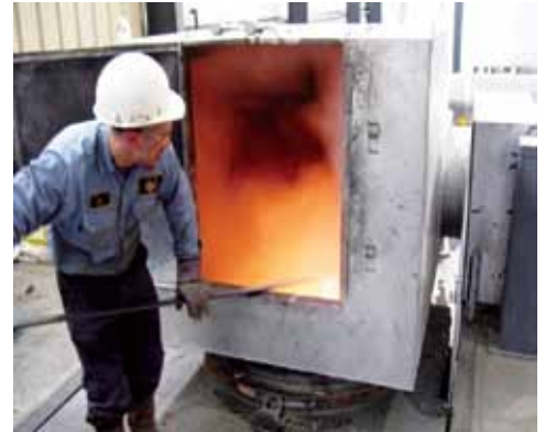
Melting furnaces operating at 2,300 degrees Fahrenheit.
