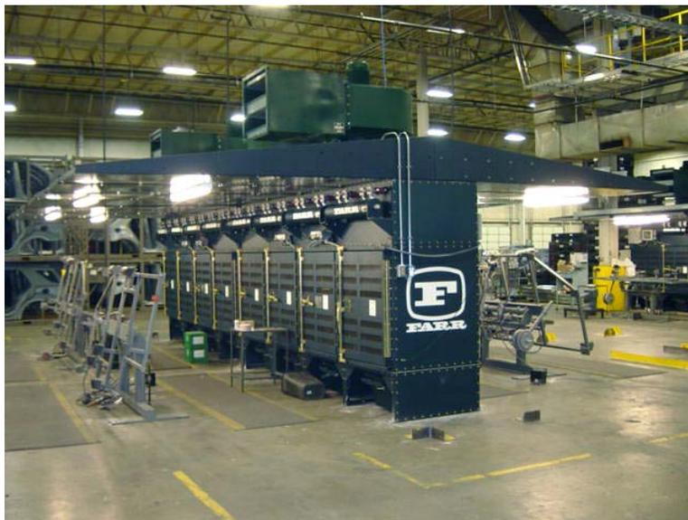
More specifically, eight filter modules, some customized roof panels and modular accessories would make up the four separate GSB's. Two would install side by side against the back wall of the work area. Between them, four more GSB's would be configured "double-sided," drawing air from both sides and further reducing the amount of used floor space.
