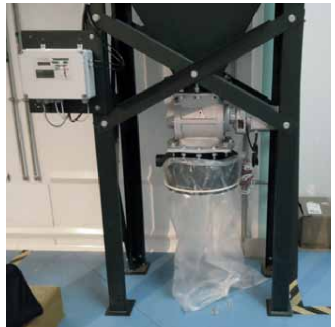
Dust removal is quick and simple with the rotary valve which discharges to a heavy duty plastic bag.
