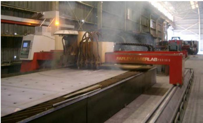
Before the Farr Gold Series® collector was installed smoke from plasma cutting operation filled the facility.
