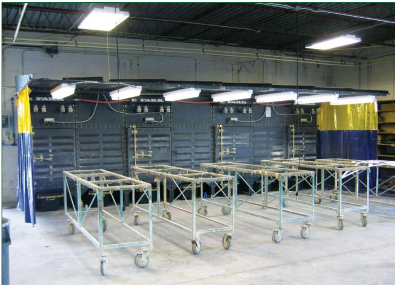
*21,600 CFM Gold Series Booth encapsulates blast dust in countertop manufacturing area.*
